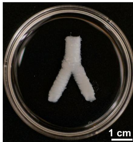
**Figure S3 | Y-shaped bioprinted branched vessel in high resolution.**
