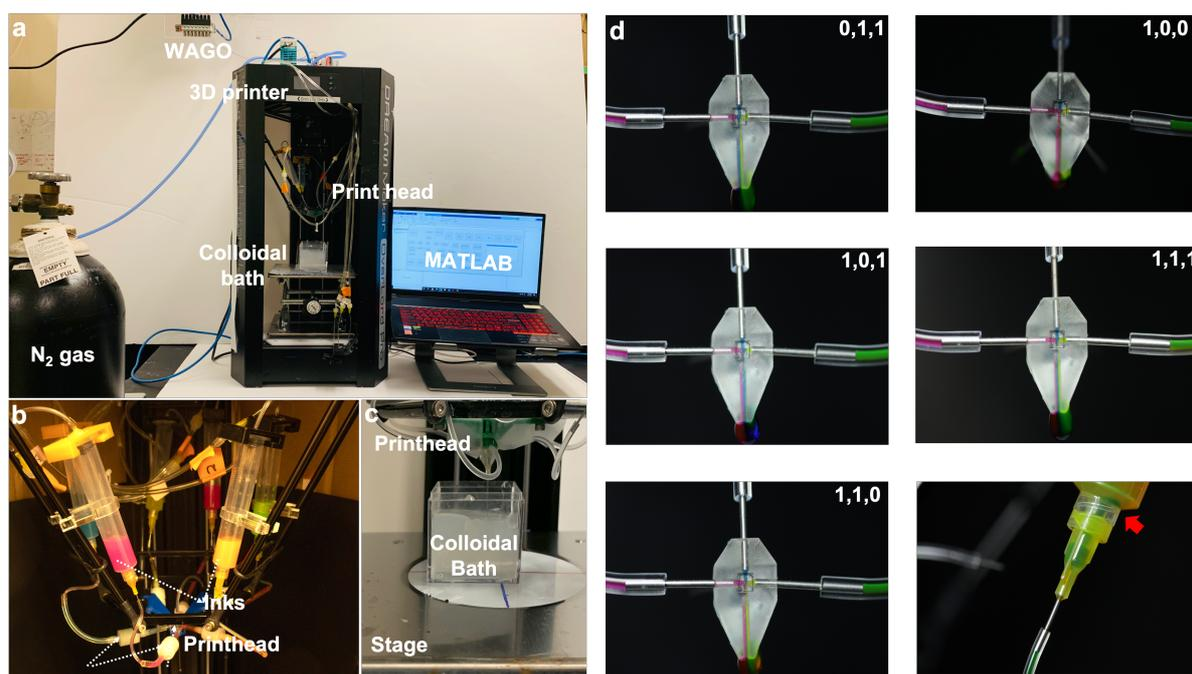
**Figure S1 | M<sup>3</sup> system.** **a**, Photograph showing different components of the printing system. **b**, Close-up of different ink syringes (6 in this case) feeding into the single nozzle printhead via check valves. **c**, colloidal bath sitting on a stage where printing happens. and **d**, Effect of check valve on ink mixing when opened (1) or closed (0) for Red (R), Green (G), and Blue (B), respectively. Binary codes are sequentially for RGB inks.
