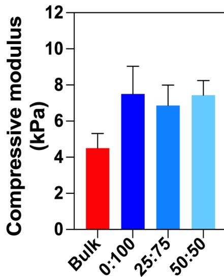
**Figure S7 | Compressive modulus of GCGs.** Compressive moduli of GCGs with different gelatin: GelMA ratio (gelatin: GelMA = 0:100, 25: 75, and 50:50).
