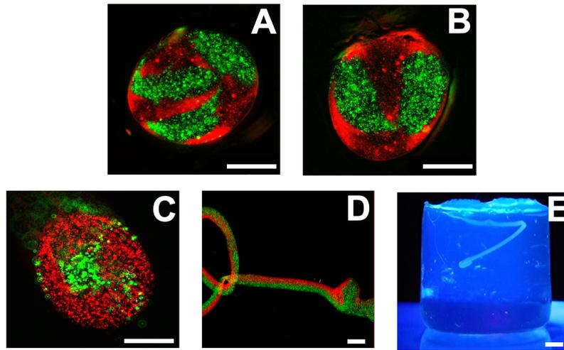
**Figure S2 | Unique printing shapes from  $M^3$ .** **a**, basket shape, **b**, insect eye, **c**, solid donut with green core and red shell, **d**, knot, **e**, serpentine shapes, respectively. Scale bars=500  $\mu\text{m}$ .
