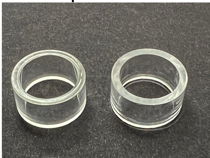
SF9A. Glass chambers. Left (fire polished side up). Right (ground glass side up).
