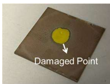
Fig. R1-3. The STPW was damaged by the water droplet.
