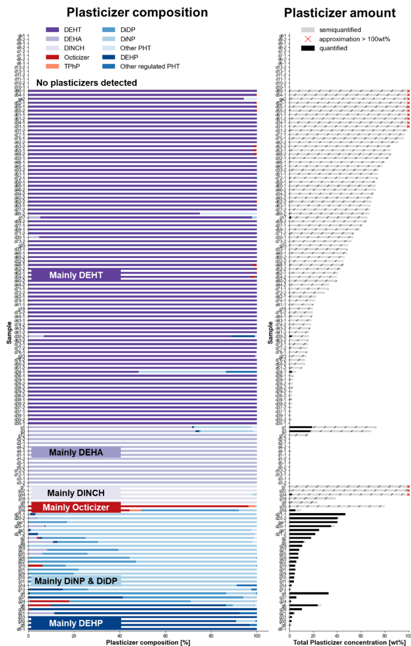
Figure S9: Plasticizer composition (left) and amount (right) by sample. Sorted by the major plasticizer per sample. Semi quantification of some plasticizer resulted in very high concentration estimates (some concentrations are even above 100wt%), which is mainly due to calibration curve uncertainty especially for signals above the calibration curve range.
