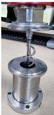
Figure S23. Custom-made reactor used for blending.
