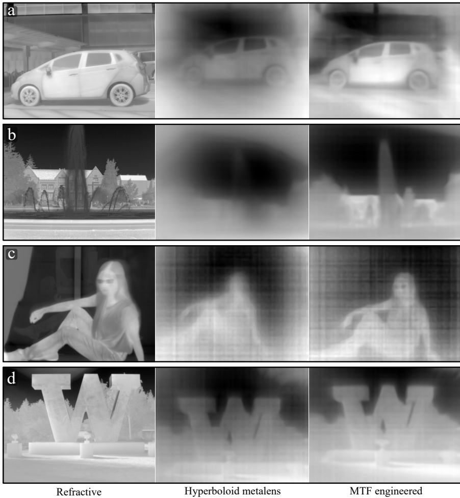
Fig. S6 LWIR imaging “in the wild”. Four scenes are imaged using the refractive LWIR lens (left), the hyperboloid metalens (middle), and the MTF engineered meta-optic with complex scatterers (right). The four scenes were all captured during daytime on a sunny day depicting (a) a parked car on a sunny day; (b) a fountain in the foreground against a building in the background; (c) a woman resting against a window; (d) a metallic structure.
