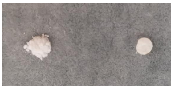
Fig. R10 The image of (\text{CH}_3-(\text{CH}_2)_9)_2\text{NH}_2\text{Cl} samples after the pressurization of 100 MPa at room temperature (left) and 330 K (right).
