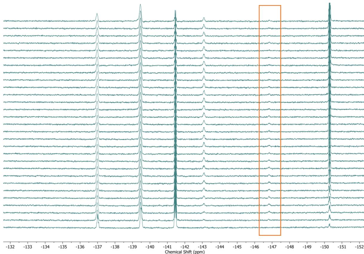
**Figure S20.** Zoom in of  $^{19}\text{F}$  NMR data of a sample enriched with ( $E_MZ_M$ )-**1** upon irradiation to PSS with 455 nm light at  $-85\text{ }^\circ\text{C}$  in  $\text{CD}_2\text{Cl}_2$  (spectra taken every 5 min.). The initial spectrum (bottom spectrum) contains a mixture of ( $E_MZ_M$ )-**1**, ( $E_SZ_S$ )-**1** and ( $E_SE_S$ )-**1**. The orange box highlights the changes of the signal at  $\pm 146.8$  ppm (the signal of ( $E_SE_M$ )-**1**).
