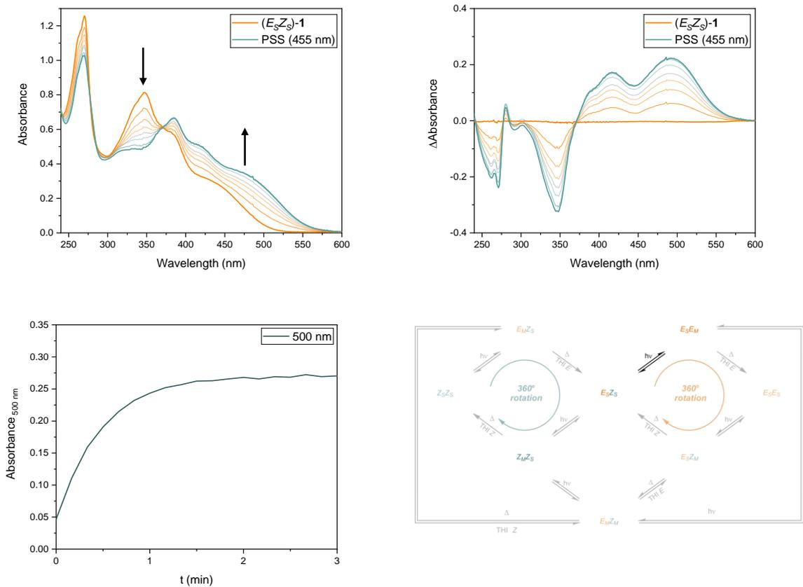
**Figure S9.** UV/Vis absorption spectra (top left) and difference spectra (top right) of  $(E_sZ_s)$ -1 in  $\text{Et}_2\text{O}$  ( $4 \times 10^{-5} \text{ M}$ ,  $-110^\circ \text{C}$ ) upon irradiation with 455 nm light. The pure isomer is shown in orange and the obtained PSS in blue. An isosbestic point is maintained at 371 nm. The absorbance at 500 nm over time upon irradiation with 455 nm light (bottom left). Motor operation overview under these conditions (bottom right).
