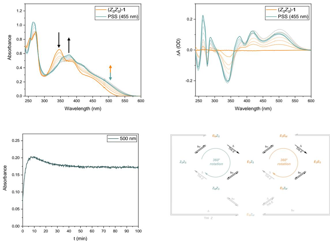
**Figure S4.** UV/Vis absorption spectra (top left) and difference spectra (top right) of (ZsZs)-1 in CH<sub>2</sub>Cl<sub>2</sub> ( $4 \times 10^{-5}$  M, -90 °C) upon irradiation with 455 nm light. The pure isomer is shown in orange and the obtained PSS in blue. The absorbance at 500 nm over time upon irradiation with 455 nm light (bottom left). Motor operation overview under these conditions (bottom right).
