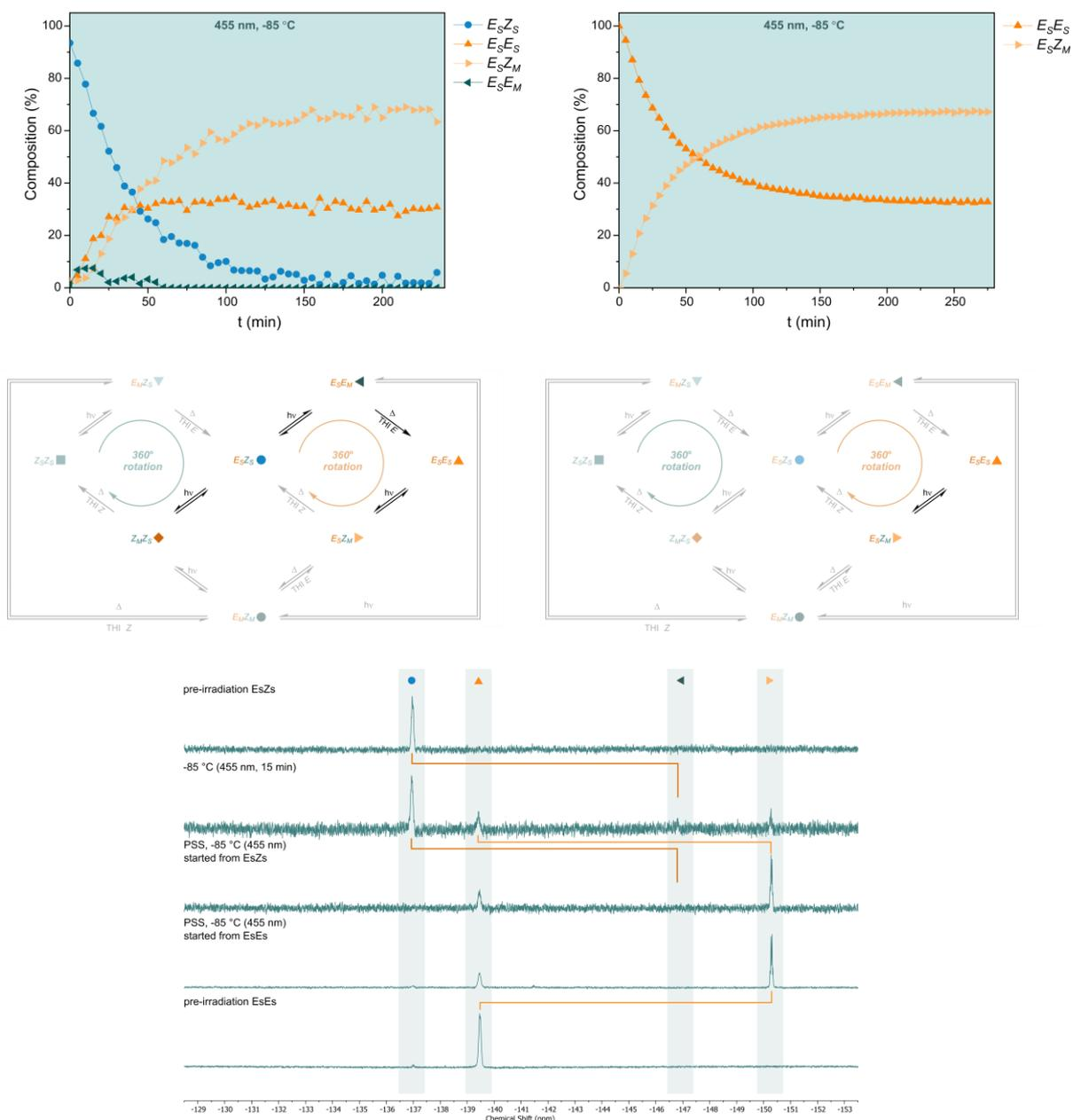
**Figure S16.** Top left: Sample of  $(EsZs)-1$  irradiated to PSS with 455 nm at  $-85\text{ }^\circ\text{C}$ . Top right: Sample of  $(EsEs)-1$  irradiated to PSS with 455 nm at  $-85\text{ }^\circ\text{C}$ . Middle: Motor operation overview under these conditions. Bottom: The corresponding  $^{19}\text{F}$  NMR spectra (470 MHz,  $-85\text{ }^\circ\text{C}$ ) of  $(EsZs)-1$  (5 mM in  $\text{CD}_2\text{Cl}_2$ ) and  $(EsEs)-1$  (11 mM in  $\text{CD}_2\text{Cl}_2$ ).
