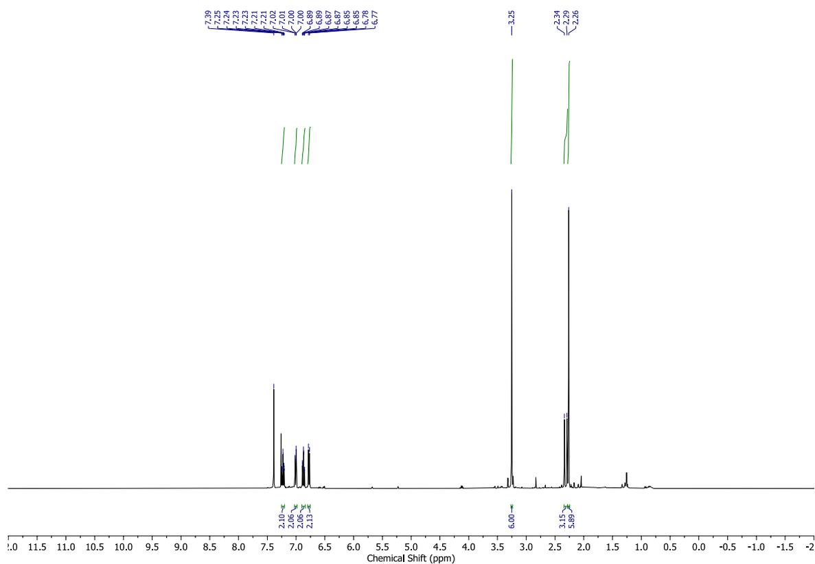
Figure S34.  $^1\text{H}$  NMR spectrum of  $(Z_sZ_s)\text{-1}$  ( $\text{CDCl}_3$ , 20 °C).
