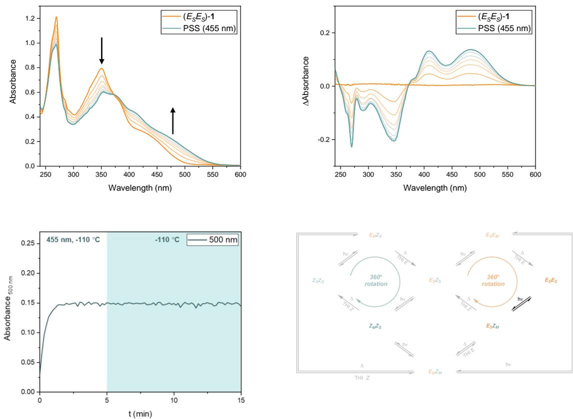
**Figure S11.** UV/Vis absorption spectra (top left) and difference spectra (top right) of  $(E_sE_s)$ -1 in Et<sub>2</sub>O ( $4 \times 10^{-5}$  M, -110 °C) upon irradiation with 455 nm light. The pure isomer is shown in orange and the obtained PSS in blue. An isosbestic point is maintained at 372 nm. The absorbance at 500 nm over time upon irradiation with 455 nm light (5 min) and in the dark (10 min) (bottom left). Motor operation overview under these conditions (bottom right).
