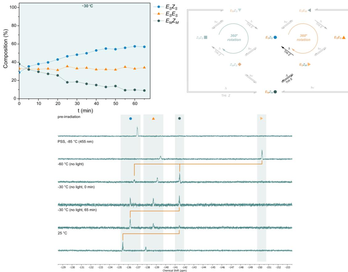
**Figure S17.** Left: Thermal decay of pre-irradiated ( $Z_5E_5$ )-**1** (PSS with 455 nm at -85 °C) at -30 °C (65 min). Right: Motor operation overview under these conditions. Bottom: The corresponding  $^{19}\text{F}$  NMR spectra (470 MHz, 5 mM in  $\text{CD}_2\text{Cl}_2$ ) of **1** recorded at the labelled temperatures.
