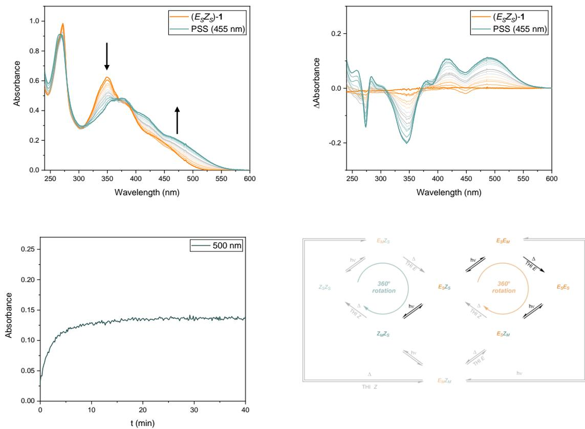
**Figure S5.** UV/Vis absorption spectra (top left) and difference spectra (top right) of  $(E_S Z_S)$ -1 in  $\text{CH}_2\text{Cl}_2$  ( $4 \times 10^{-5}$  M,  $-90$  °C) upon irradiation with 455 nm light. The pure isomer is shown in orange and the obtained PSS in blue. The absorbance at 500 nm over time upon irradiation with 455 nm light (bottom left). Motor operation overview under these conditions (bottom right).
