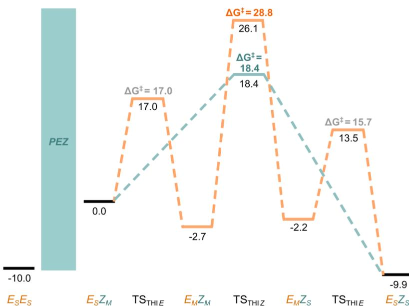
**Figure S33.** Thermal conversion of ( $E_S Z_M$ )-**1** to ( $E_S Z_S$ )-**1** via pathways A (THIZ shown in orange) and B (a series of CO-flip (THIE) and THIZ and THIE shown in blue). For transition states, the activation barriers are referenced to the associated initial state. Energies (black) and activation barriers (bold coloured) were calculated at the  $r^2$ SCAN-3c CPCM(CH<sub>2</sub>Cl<sub>2</sub>) level of theory and are shown in kcal mol<sup>-1</sup>.
