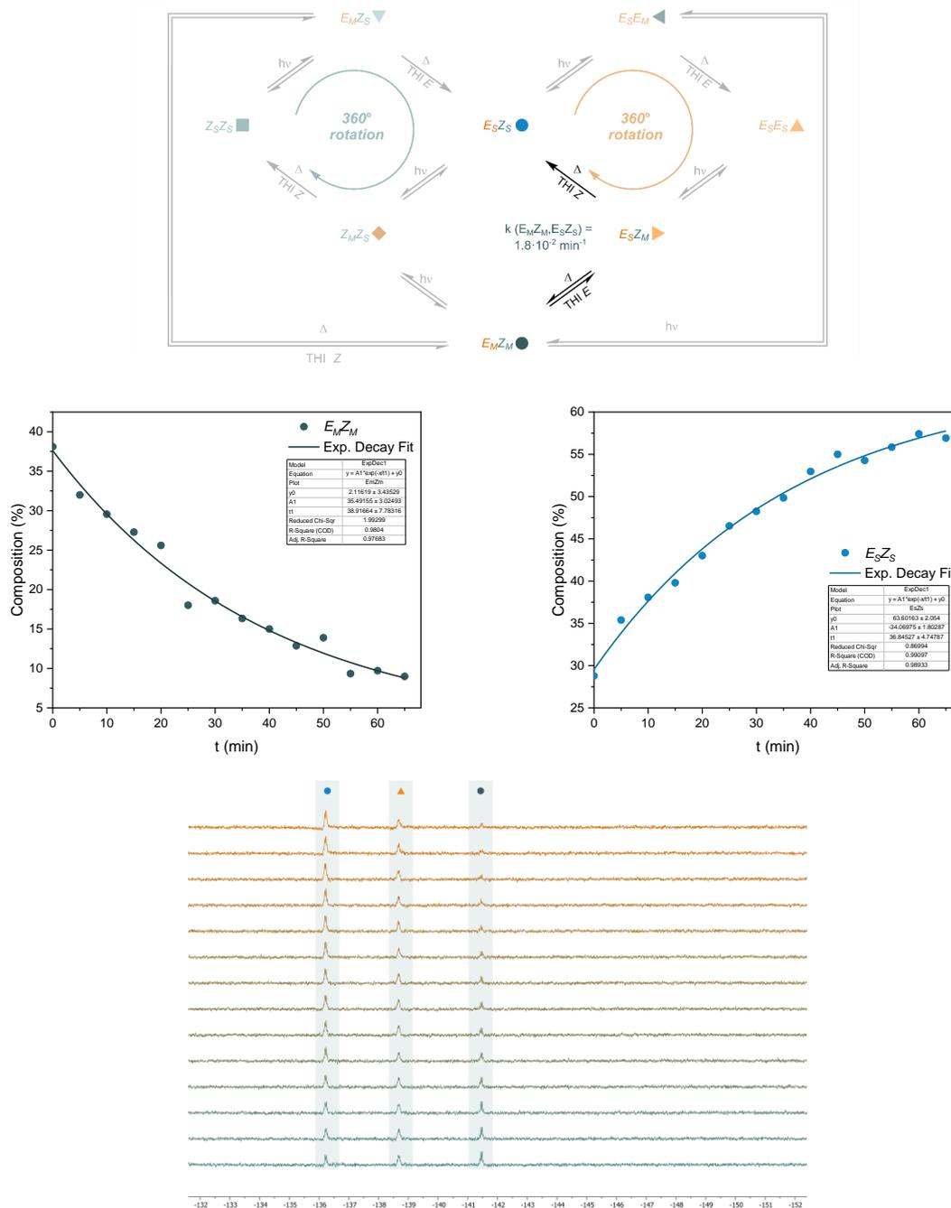
**Figure S28.** Proposed mechanism with rate constants (top). The trace of  $(E_MZ_M)$ -1 (middle left) and  $(E_SZ_S)$ -1 (middle right) in the thermal decay of pre-irradiated  $(Z_S E_S)$ -1 (PSS with 455 nm at  $-85\text{ }^\circ\text{C}$ ) at  $-30\text{ }^\circ\text{C}$  versus time. The half-life ( $t_{1/2}$ ) was obtained by fitting the data to the mono-exponential decay equation:  $A = y_0 + A_1 e^{-t/(t_{1/2})}$  using Origin software. Stacked NMR data (bottom).
