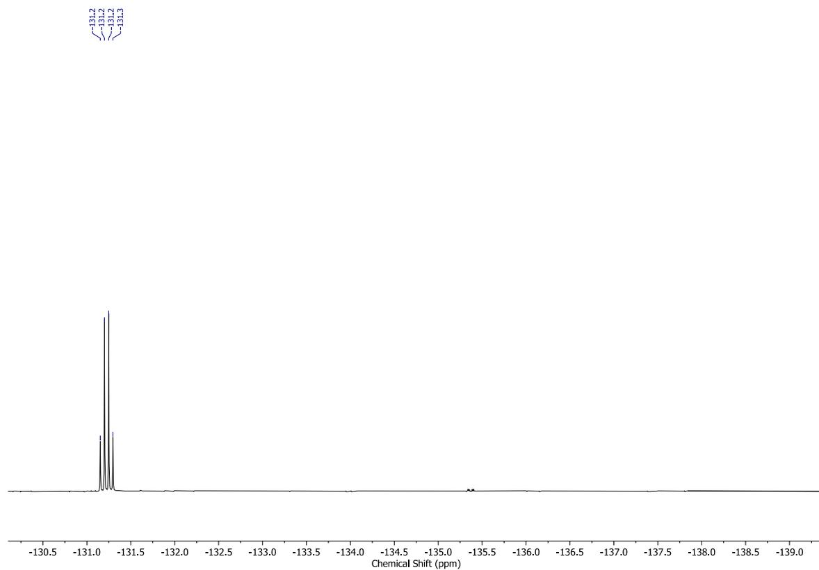
**Figure S36.**  $^{19}\text{F}$  NMR spectrum of  $(Z_5Z_5)\text{-1}$  ( $\text{CDCl}_3$ ,  $20^\circ\text{C}$ , full (top) and zoomed (bottom)).
