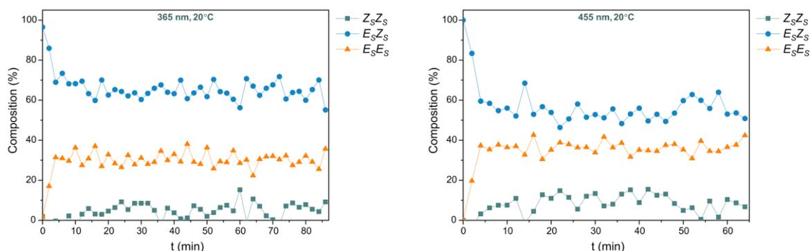
**Figure S22.** Composition over time of a sample of (*E<sub>S</sub>Z<sub>S</sub>*)-**1** in  $\text{CD}_2\text{Cl}_2$  irradiated to PSS with 365 nm (left) or 455 nm (right) at 20 °C followed by  $^{19}\text{F}$  NMR spectroscopy (470 MHz).
