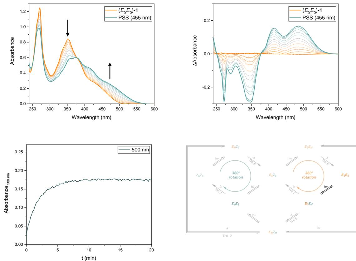
**Figure S6.** UV/Vis absorption spectra (top left) and difference spectra (top right) of  $(E_sE_s)\text{-1}$  in  $\text{CH}_2\text{Cl}_2$  ( $4 \times 10^{-5}$  M,  $-90$  °C) upon irradiation with 455 nm light. The pure isomer is shown in orange and the obtained PSS in blue. An isosbestic point is maintained at 378 nm. The absorbance at 500 nm over time upon irradiation with 455 nm light (bottom left). Motor operation overview under these conditions (bottom right).
