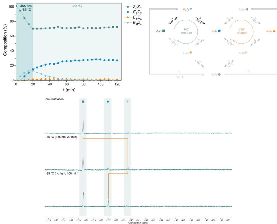
**Figure S18.** Left: Thermal decay of pre-irradiated ( $Z_S Z_S$ )-**1** (455 nm for 20 min at -85 °C) at -85 °C. All measurements were performed at -85 °C. Right: Motor operation overview under these conditions. Bottom: The corresponding  $^{19}F$  NMR spectra (470 MHz, -85 °C, 5 mM in  $CD_2Cl_2$ ) of **1**.
