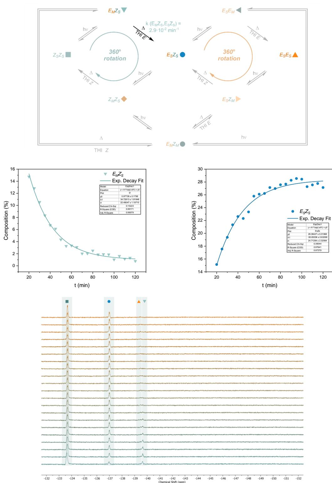
**Figure S27.** Proposed mechanism with rate constants (top). The traces of ( $E_MZ_S$ )-1 (left middle) and ( $E_SZ_S$ )-1 (right middle) in the thermal decay of pre-irradiated ( $Z_SZ_S$ )-1 (455 nm for 20 min at  $-85\text{ }^\circ\text{C}$ ) at  $-85\text{ }^\circ\text{C}$  versus time. The half-life ( $t_{1/2}$ ) was obtained by fitting the data to the mono-exponential decay equation:  $A = y_0 + A_1 e^{-t/(t_{1/2})}$  using Origin software. Stacked NMR data (bottom).
