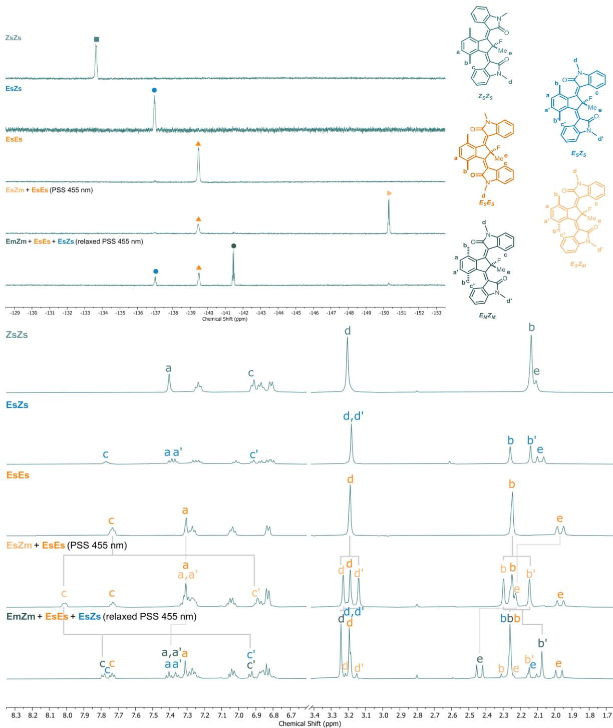
**Figure S14.** Top:  $^{19}\text{F}$  NMR spectra (470 MHz,  $-85^\circ\text{C}$ ,  $\text{CD}_2\text{Cl}_2$ ) of  $(ZsZs)$ -1,  $(EsZs)$ -1,  $(EsEs)$ -1, a sample enriched with  $(EsZm)$ -1, and a sample enriched with  $(EmZm)$ -1. Bottom:  $^1\text{H}$  NMR spectra (500 MHz,  $-85^\circ\text{C}$ ,  $\text{CD}_2\text{Cl}_2$ ) of  $(ZsZs)$ -1,  $(EsZs)$ -1,  $(EsEs)$ -1, a sample enriched with  $(EsZm)$ -1, and a sample enriched with  $(EmZm)$ -1. Key signals are assigned with letters.
