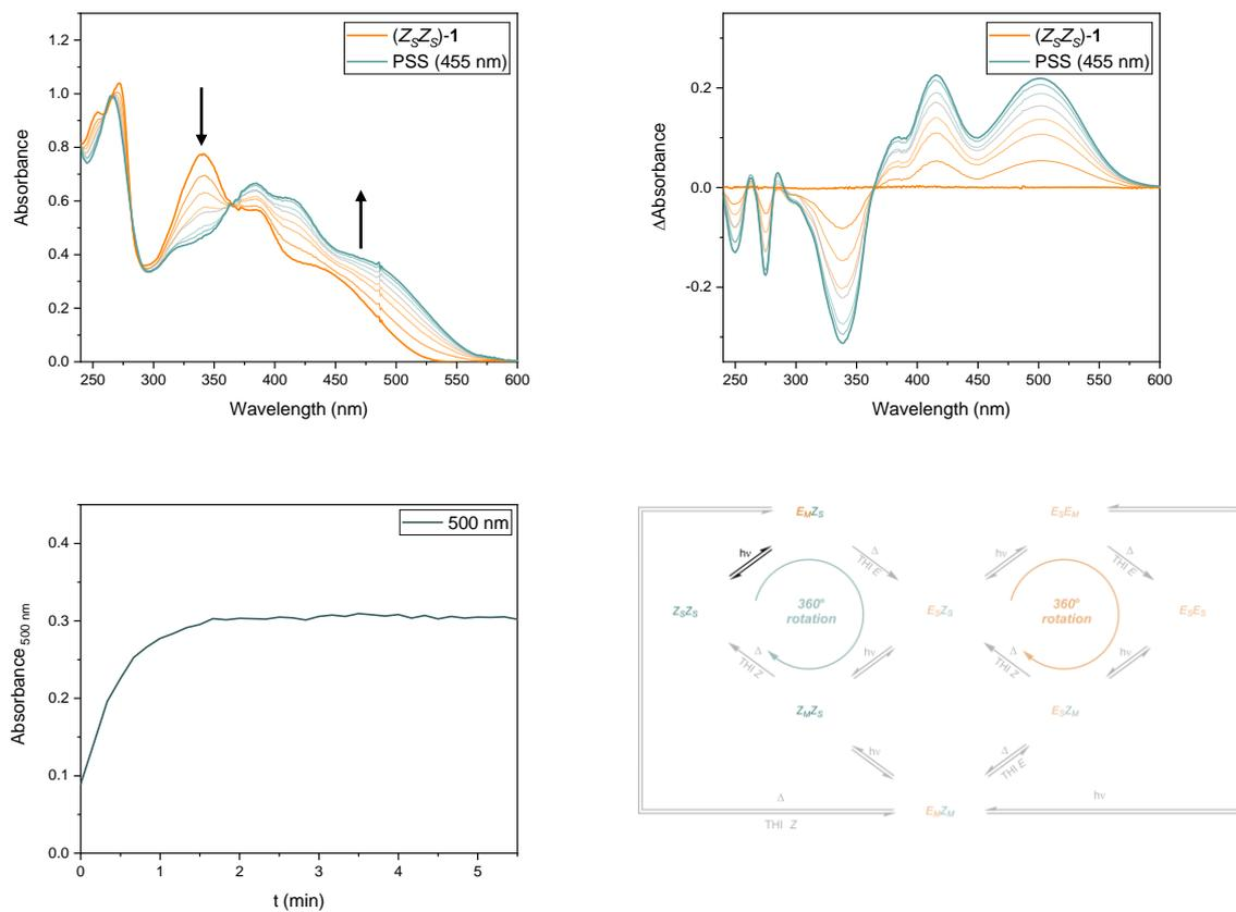
**Figure S7.** UV/Vis absorption spectra (top left) and difference spectra (top right) of  $(Z_sZ_s)$ -1 in  $\text{Et}_2\text{O}$  ( $4 \times 10^{-5}$  M,  $-110$  °C) upon irradiation with 455 nm light. The pure isomer is shown in orange and the obtained PSS in blue. An isosbestic point is maintained at 365 nm. The absorbance at 500 nm over time upon irradiation with 455 nm light (bottom left). Motor operation overview under these conditions (bottom right).
