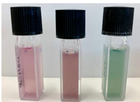
Figure S15. Photographs of PCN-223 suspended in acetone, water and 0.01 M HCl from left to right.
