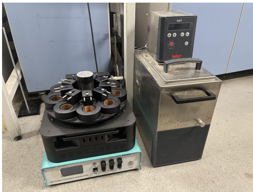
Figure S1 PCX-50C multi-channel photochemical reaction system (Beijing Perfectlight) and cooling bath thermostat.
