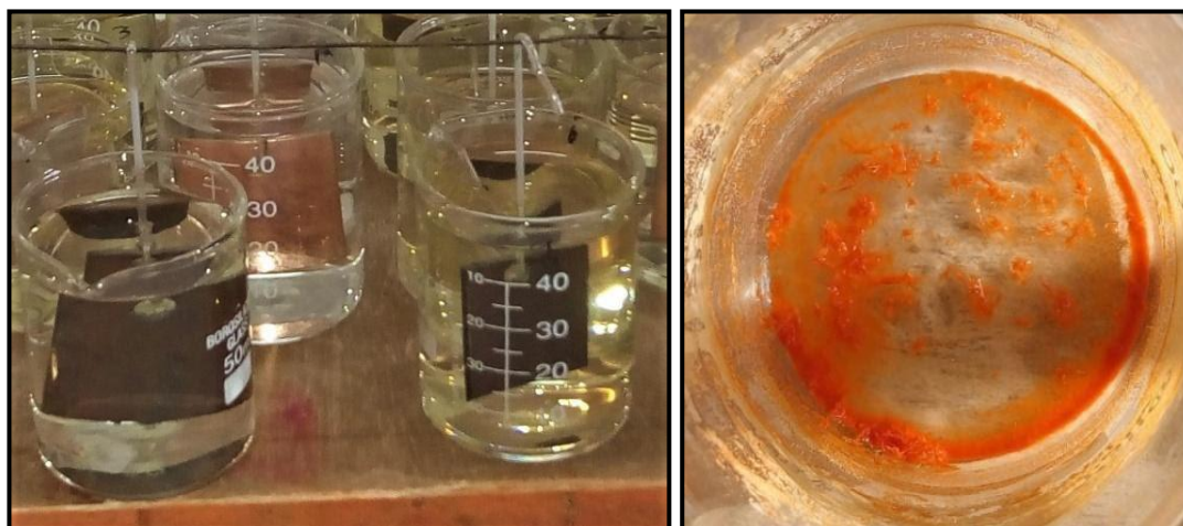
Figure S7: Weight loss measurement process and fresh crystals of 4-[(4-Nitrobenzylidene)-amino]-antipyrine (4-NBAAP).
