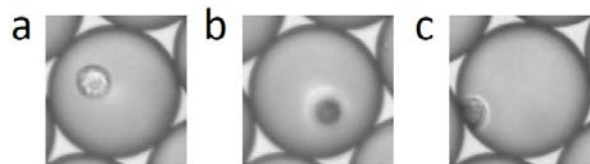
The same cell inside the droplet (a) at the focal plane, (b) out of the focal plane, and (c) near the interface.
