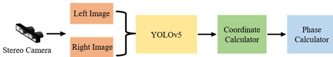
Figure. S41. The architecture of object detection and localization.
