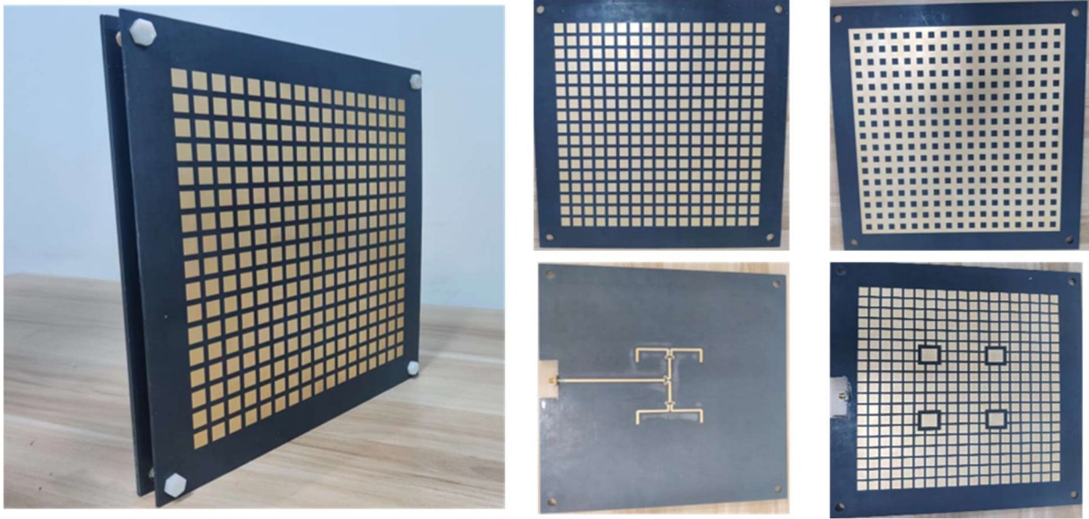
Figure. S4. The fabricated NFF with profile of \lambda/4
