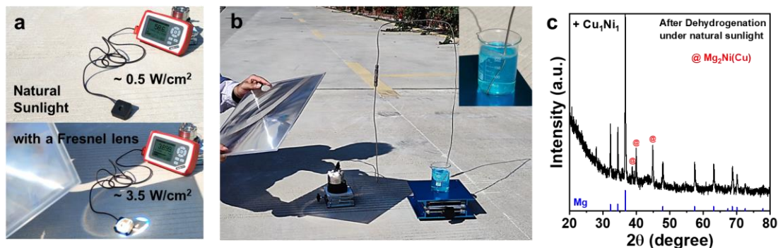
Supplementary Figure 22. Outdoor experiment by natural solar. a) Light intensity of natural solar without and with a commercial PMMA Fresnel lens. b) H 2 desorption experiment using natural solar as the energy source. The inset image shows the enlarged hydrogen bubbles. c) XRD patterns of the sample pellet after H 2 desorption under natural light. The unit a.u. means to arbitrary units. Source data are provided as a source data file.
