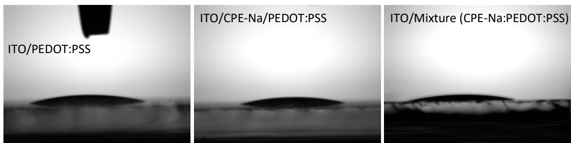
Figure S2. Contact angle for a drop of PM6:Y7 on the prepared layers. The mean angles are summarized in Table S2 .
