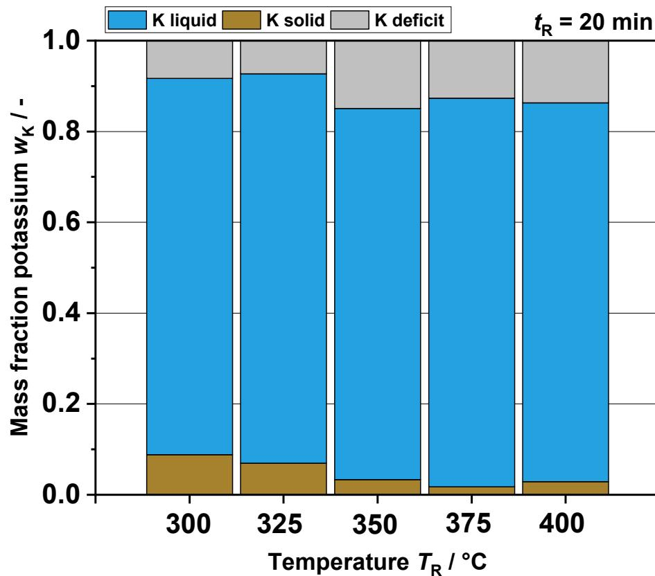
Figure S4. Potassium mass balance at different reaction temperatures  $T_R$
