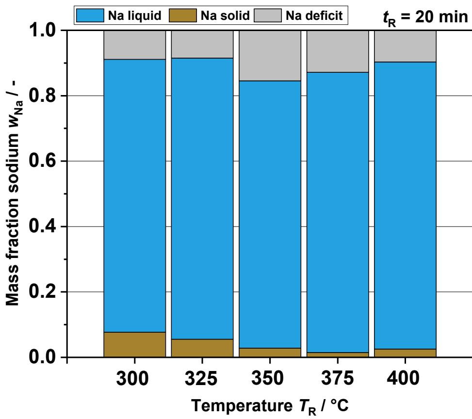
Figure S3. Sodium mass balance at different reaction temperatures  $T_R$
