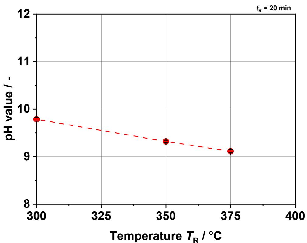
Figure S1. pH values for the liquid product after HTL of BL at three different reaction temperatures
