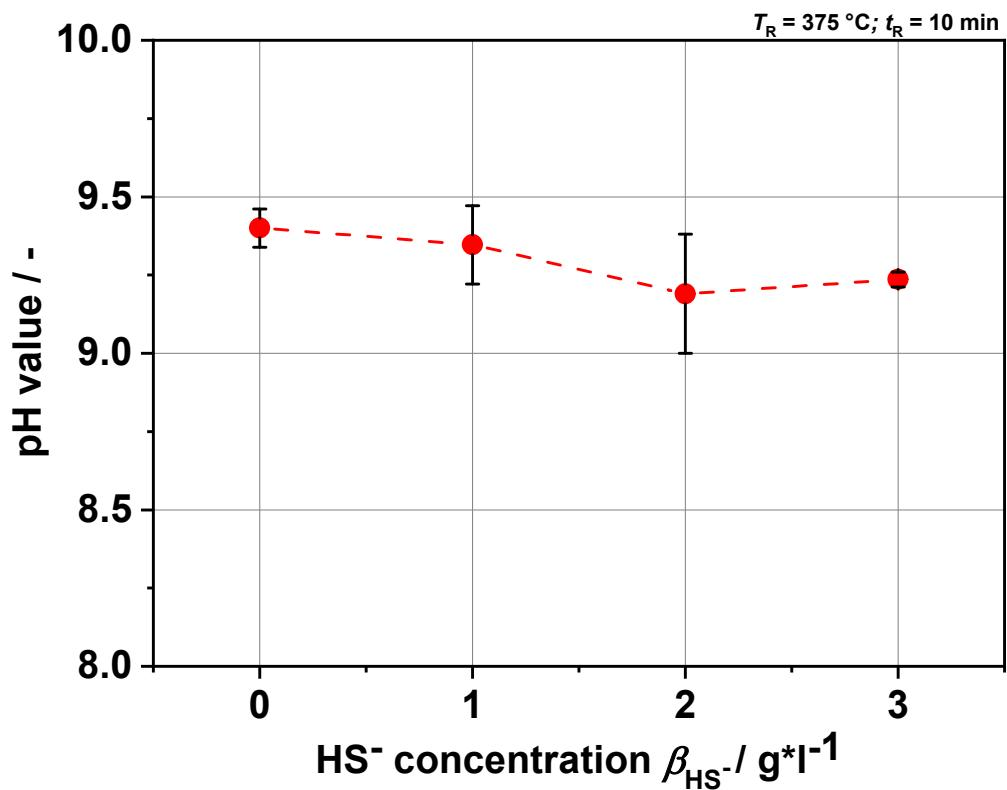
Figure S2. pH values for the liquid product after HTL of MBL at  $T_R = 375 \text{ } ^\circ\text{C}$  and  $t_R = 10 \text{ min}$  with different HS<sup>-</sup> feedstock concentrations
