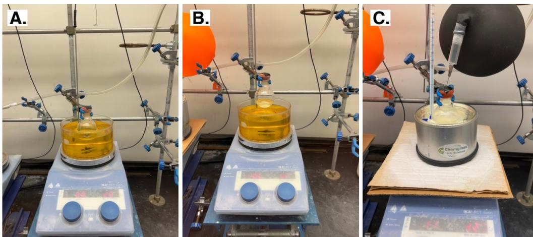
**Graphical set-up 1:** One-pot transformation of chiral *N,N*-diisopropyl urea protected *tert*-butyl sulfoximines to sulfinyl ureas. **A.** Reduction of *t*-butyl sulfoximines via de-*tert*-butylation using *t*-BuOK, heating at  $80^{\circ}\text{C}$  in THF. **B.** Cooling to room temperature after 2 hours at  $80^{\circ}\text{C}$ . **C.** Cooling to  $-20^{\circ}\text{C}$  and quenching with AcOH (2 eq.) followed by addition of NFSI (1 eq.).
