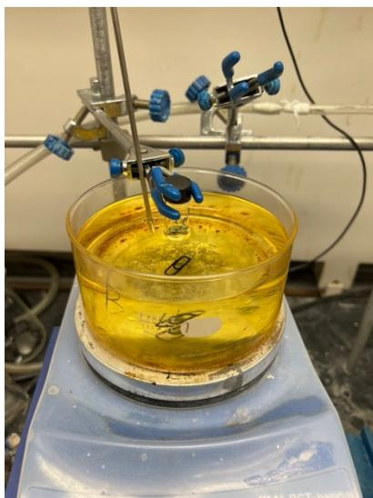
**Graphical set-up 2:** Deprotection of *N,N*-diisopropyl sulfonimidoyl ureas to *N*-H sulfonimidoyl groups using CSA in HFIP at 70 °C.
