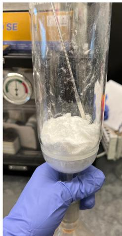
**Image 1:** Filtration of *tert*-butyl phenyl sulfoximine **2a** after first crop of recrystallization.
