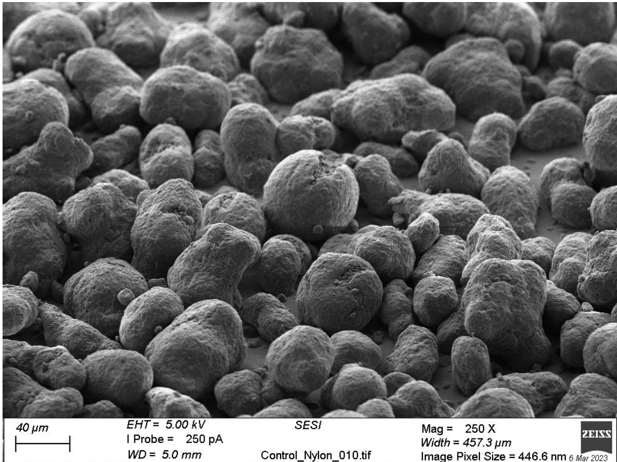
Supplementary Fig 23 - SEM of commercial virgin PA-12 (uncoated) showing the characteristic 'potato' shape and the range of particles sizes that are present in the commercial sample.
