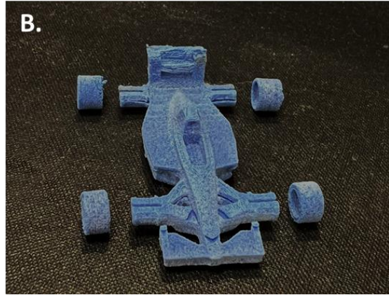
S55 – Printed race car model built from a 80/20 mix of virgin PA-12 and PA-12 coated with P(IBMA-DB3MA) respectively. A.) fully assembled. B.) with detachable wheels removed.
