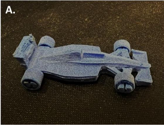
S55 – Printed race car model built from a 80/20 mix of virgin PA-12 and PA-12 coated with P(IBMA-DB3MA) respectively. A.) fully assembled. B.) with detachable wheels removed.
