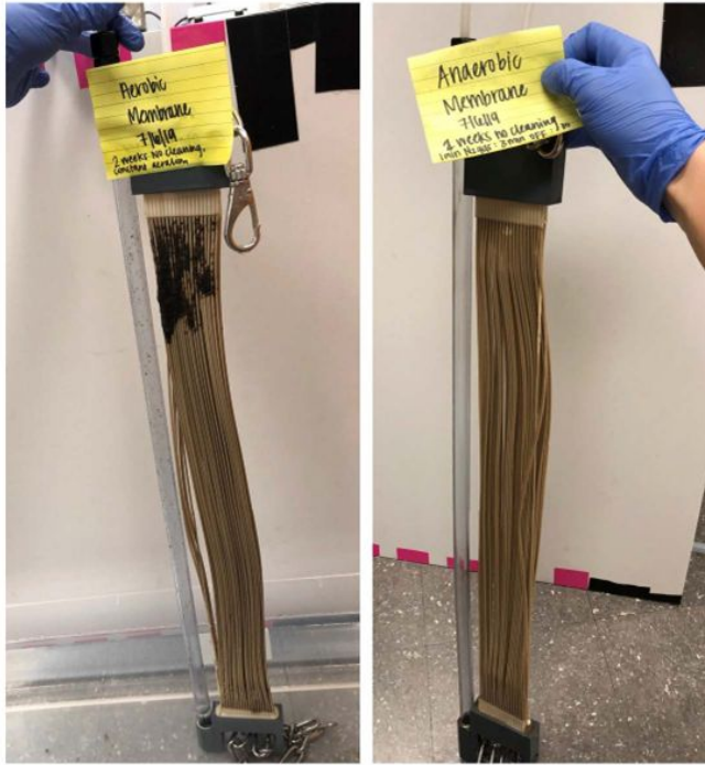
Figure S1. Aerobic (left) and anaerobic (right) membranes, before cleaning, after running two treatment cycles on 100% municipal wastewater.
