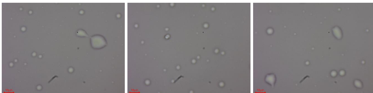
Figure S16. Microscope images of 0.25M Toluene in SOBS/H 2 O; red bars represent 10 microns
