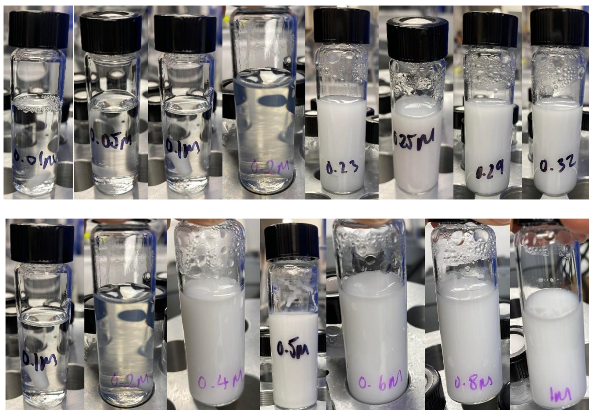
Figure S3. Physical appearance of vial containing TPGS-750-M (0.5 % w/w) and 0.01 – 1.0 M toluene in deionised water.
