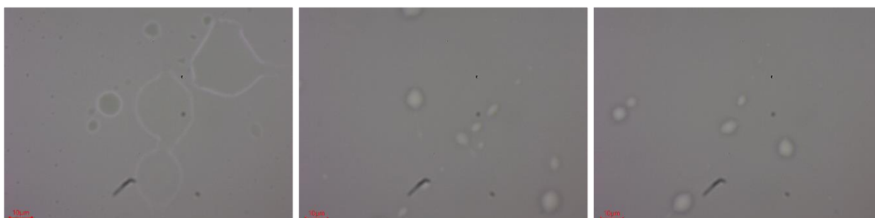
Figure S15. Microscope images of 0.25M Toluene in CPC/H 2 O; red bars represent 10 microns
