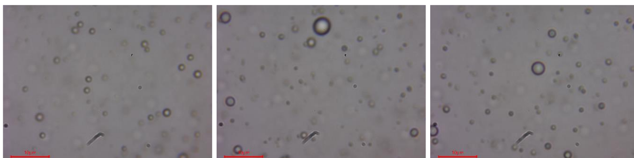
Figure S14. Microscope images of 0.25M Toluene in TPGS-750-M/H 2 O; red bars represent 10 microns
