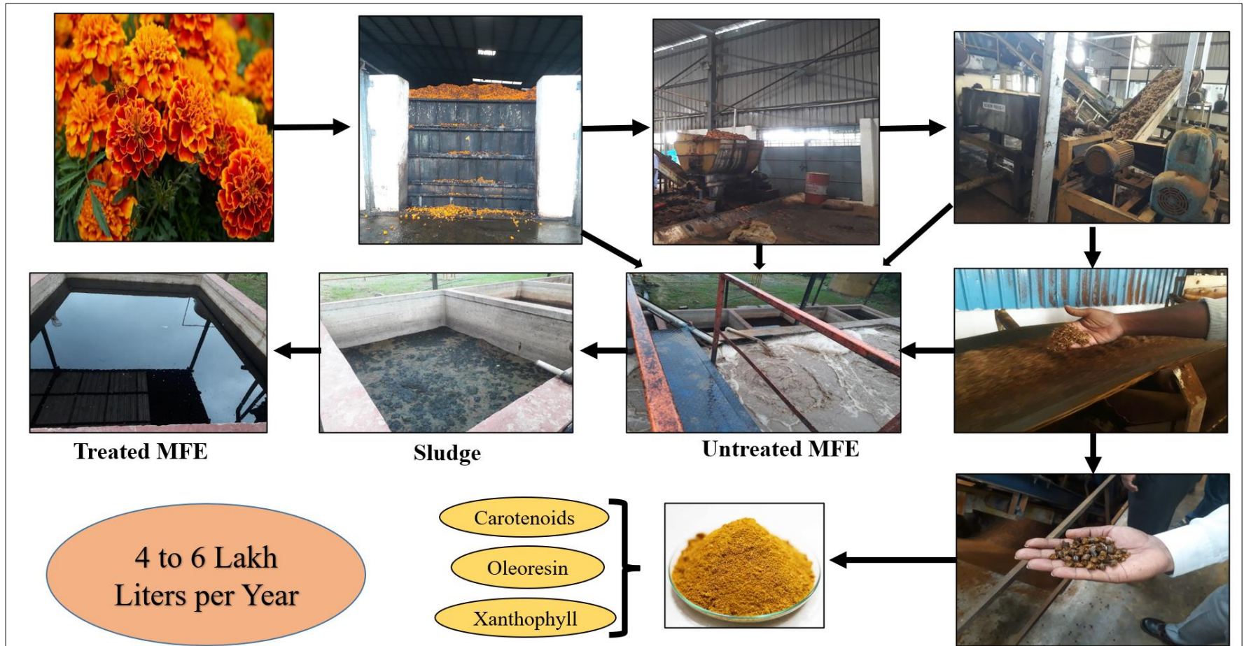
Fig. S1: Processing of marigold flowers in the industry and collection of treated and untreated marigold flower effluent (TMFE and UMFE) during the process – Flow chart: The process is as follows collecting marigold flowers, silage preparation, pressing, drying, pelletization and extraction of carotenoids, oleoresins and xanthophylls.
