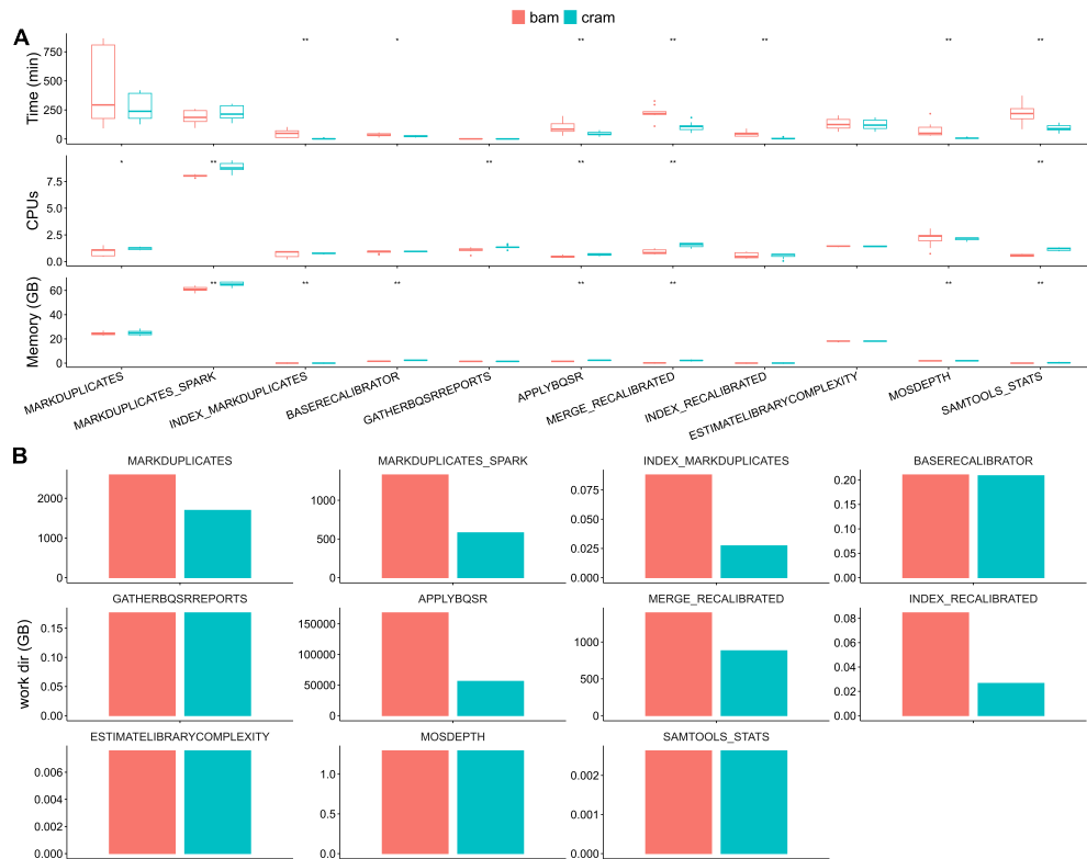
Fig. S2: Resource usage of nf-core/sarek 3.1.1 when storing intermediate data in BAM versus CRAM format for all pre-processing processes. A ): Average realtime, and maximum CPU and memory usage (peak.rss) as reported by the Nextflow trace file. For processes split within a sample (i.e. ApplyBQSR), the task with the highest runtime per sample is shown as the process runtime. Resource usage was compared using the paired Wilcoxon test (** p < 0.01 , * p < 0.05 ). Seven of the eleven processes are significantly faster when using the CRAM format. Five processes have a significantly higher CPU hour usage, and three require more memory in comparison to using BAMs. B ): Storage was evaluated by calculating the total size of the work directories of all tasks of the respective process. The storage usage between both is identical, due to Nextflow accessing the input files via symlinks. Thus only the output is measured here for each process, which is independent of input format. Each condition was repeated three times for samples of five tumor-normal paired patients.
