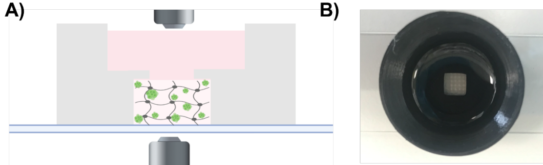
Figure S27. To measure the same sample using SERS and fluorescence imaging, a setup suitable for upright (Raman microscope) and inverted (fluorescence) microscopy was required. As such, the scaffold (with ECM and cellular components) was placed on top of a quartz glass slide or cover slip, compatible with both imaging modalities (A). To hold the scaffold in place on the slide, a 3D-printed PCL holder was designed, suppressing scaffold movement (in XYZ). The conical shape was designed to hold a significant amount of cell media (at least 1 mL) in addition to the insertion of immersion objectives (B).
