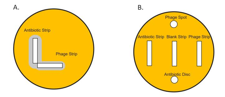
**Figure S1.** Plate configurations for screening of antibiotic-phage cooperativity. The test plate (Panel A) and control plate (Panel B) configurations are shown.
