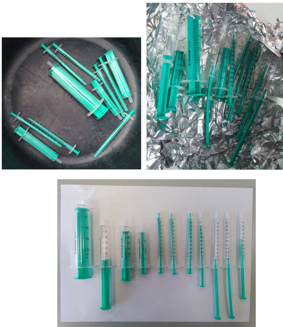
Figure S27: Syringes before (top left) and after (top right and bottom) autoclaving for reuse in a chemistry laboratory. Stains and remaining water droplets led to unfeasibility.
