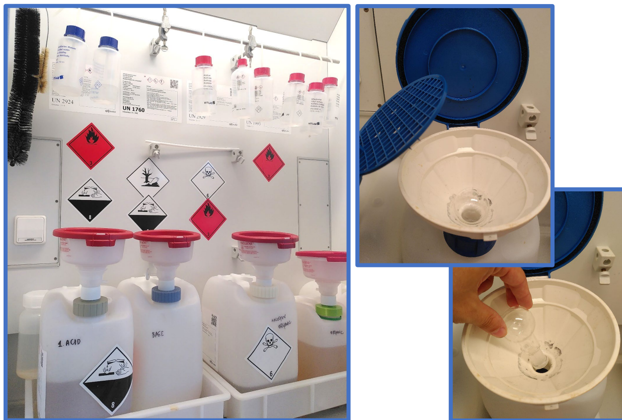
Figure S26: Funnels with lid to prevent solvent evaporation from waste canisters (left). Use of a round bottom flask to improve solvent loss by evaporation, which can serve as alternative to funnels with a lid (right). Another alternative to the round bottom flask is the plastic balls used to cover water baths in rotary evaporators, which can also be placed in a funnel to prohibit solvent loss by evaporation. Image reproduced from previously published guidebook ( https://doi.org/10.26434/chemrxiv-2023-q3lmq-v2 ).
