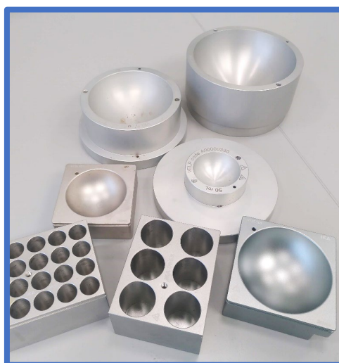
Figure S21: Metal heating block as efficient and safe replacement for oil heating baths. Image reproduced from previously published guidebook ( https://doi.org/10.26434/chemrxiv-2023-g3lmq-v2 ).
