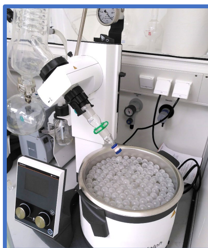
Figure S22: Plastic balls in the water bath of a rotary evaporator to prevent energy loss in form of heat. Image reproduced from previously published guidebook ( https://doi.org/10.26434/chemrxiv-2023-q3lmq-v2 ).
