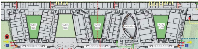
Figure S10: Design of the Feringa Building (top) including the 4 courtyards to enhance biodiversity (bottom) and solar panels (900 m 2 ), HR glass, heat pumps, automated closing fume hoods, LED and natural light.
