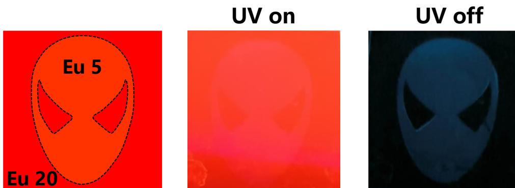
Supplementary Figure 34. The encrypted Spider-Man pattern is hidden with similar fluorescence and displayed by afterglow.
