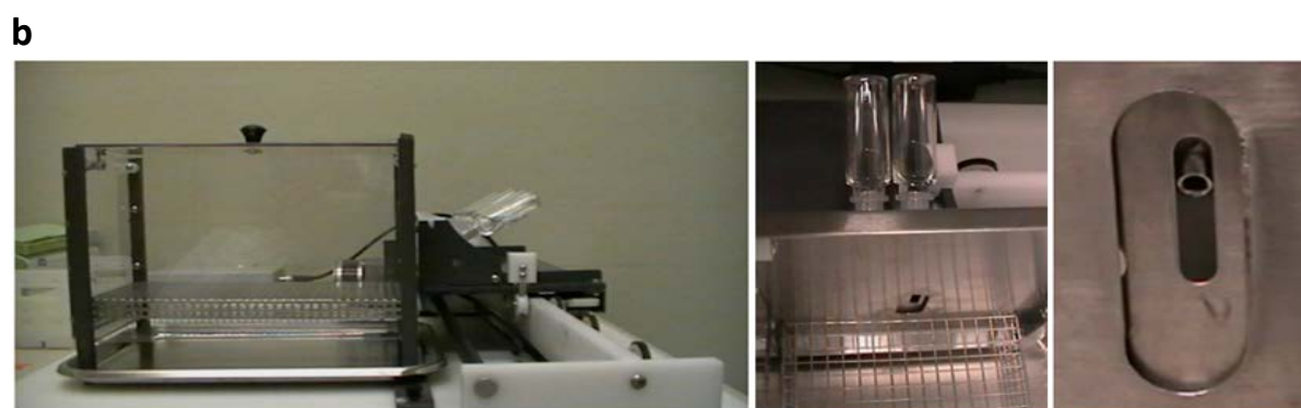
(a) Protocol and (b) setup (DavisRig lickometer) for taste preference tests.
