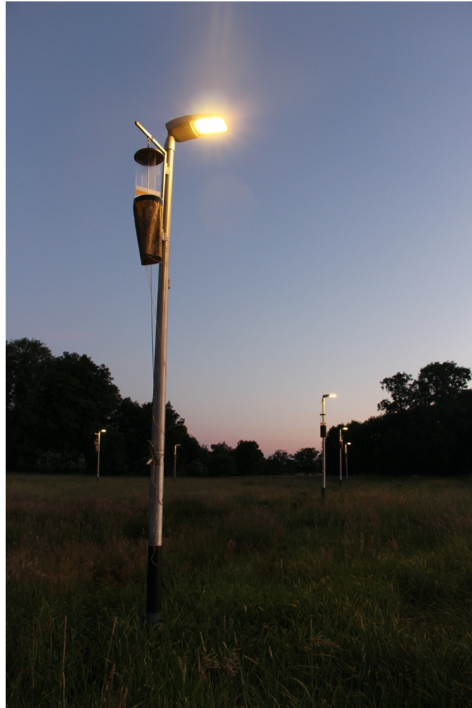
Supplementary Figure 3: Schreder Teceo LED luminaires equipped with flight interception traps on the western field of the Experimental site in Westhavelland. n=12 luminaires.
