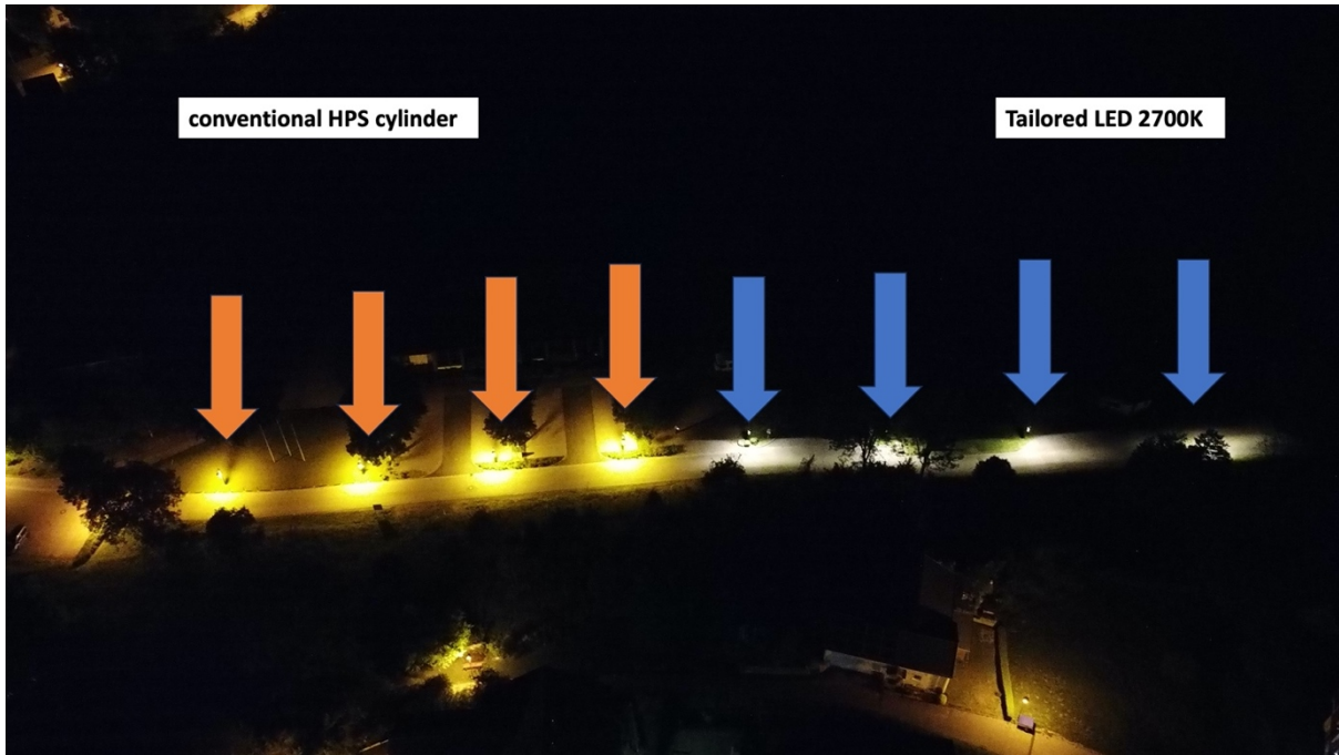
Supplementary Figure 15: Road lights at the Municipal Site Heimbachau. Tailored and shielded luminaires (LED, E_m = 5.1 \text{ lx} , CCT 2700K) n=4 (blue arrows). Conventional luminaires (HPS bow-shaped, E_m = 5.1 \text{ lx} , 2000K) n=4 (orange arrows). Photos captured by drone.
