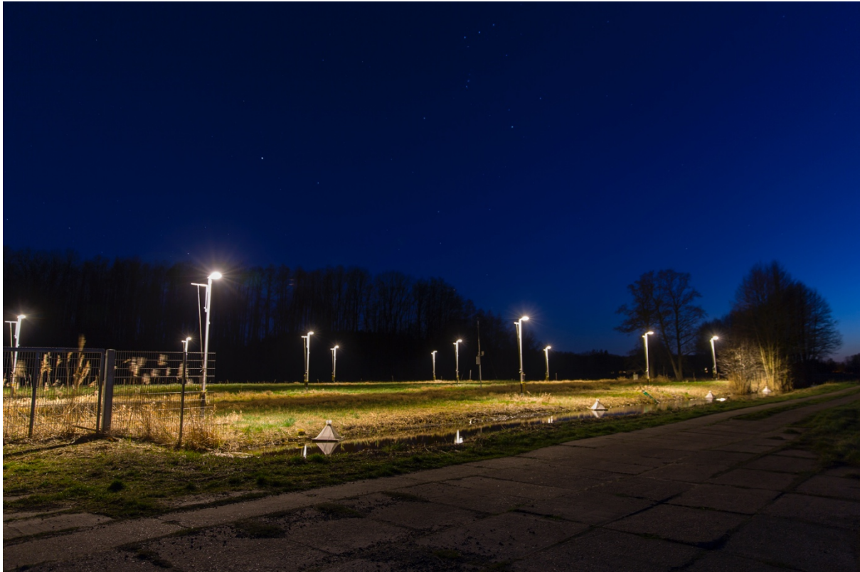
Supplementary Figure 2: Undimmed Schreder Teceo luminaires (LED, 30.6 lux, CCT 3000K) installed from 2019-2020 on the western field of the Experimental site in Westhavelland. n=12 luminaires.
