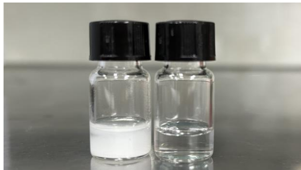
Fig. R9 The supersaturated solution (5 mg/ml) of BCP (left) and the solution filtered using a PTFE filter (right).
