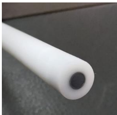
Figure S1. Optical image of Mn-TPP/RGO/GCE fabricated electrode with geometrical surface area of 0.07 cm 2 .
