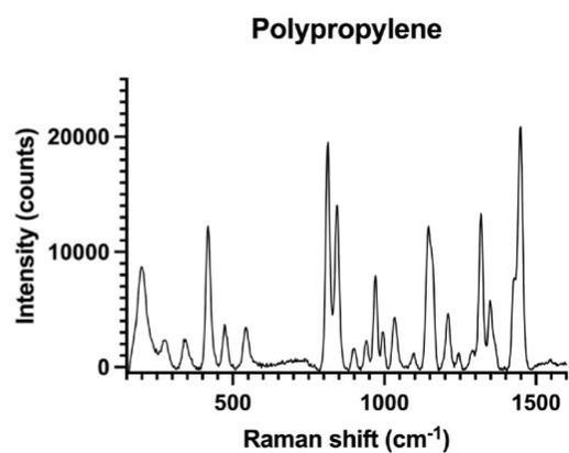
**Figure S1: Calibration standards and their corresponding Raman spectrum. (A) Sheets of pink polypropylene (PP) were placed on top of white polytetrafluoroethylene (PTFE) to create calibration standards. (B) Raman spectrum of PTFE. (C) Raman spectra of PP. Spectra were acquired using a 785 nm laser, 1s integration time.**
