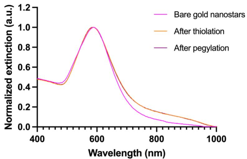
Figure S2: Extinction spectroscopy of SERRS CAs after thiolation and after PEGylation. Spectra were characterized using a UV-2600 UV-VIS spectrophotometer (Shimadzu).
