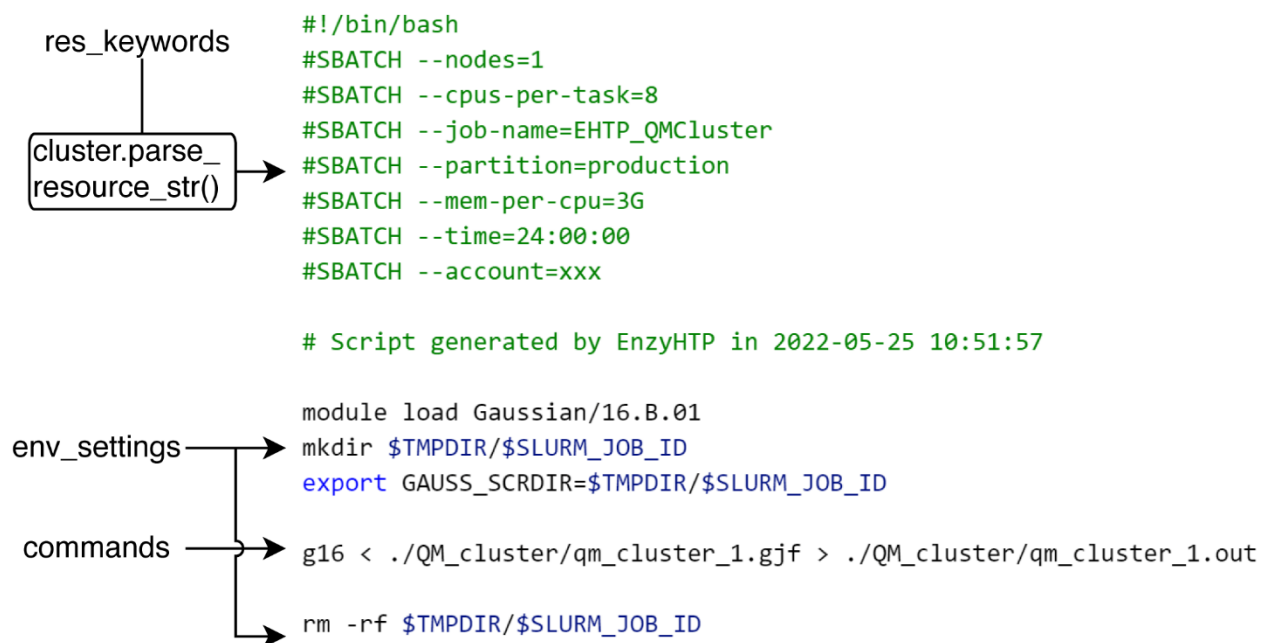
Figure S3. A sample job script that performs QM calculation using Gaussian 16. The job script is generated by the “workflow script” using commands implemented in ARMer.
