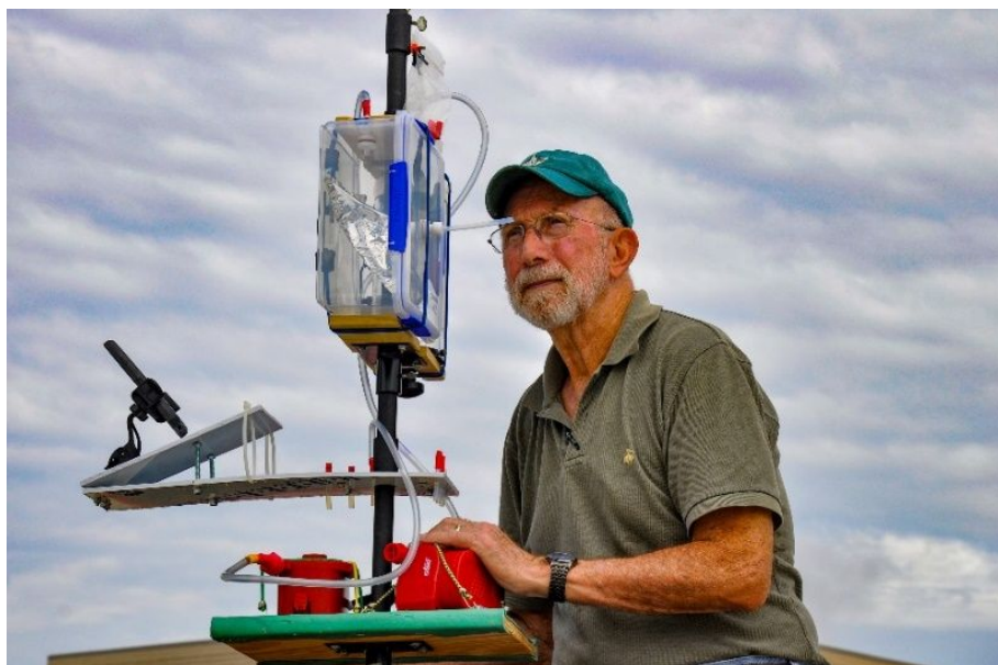
Figure S4. Second generation prototype odor-cued grab air sampling assembly. Air sample inlet located near the breathing zone of the operator. The operator observes the wind strip-indicator mast visualizing the wind direction and velocity and likely odor plume location. An m-FEP sampling bag chamber 'cartridge' and the syringe (behind the chamber) assemblies are shown rigid-mounted near the top of the pole-support assembly. A selectable vacuum/pressure air pump assembly is positioned below this syringe/bag chamber bracket assembly. A smartphone mounting platform extension is mounted between the two, positioned to permit video recording of the orientation and movement of the wind strip-indicator mast, accompanying the momentary grab sample collections. The first author is shown awaiting a characteristic odor-cue for a targeted odor event.
