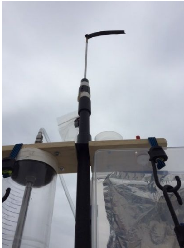
Figure S6. A smartphone captured moment-in-time of the wind strip-indicator mast orientation/wind direction is shown relative to the orientation of the sampling bag/chamber assembly. The captured video of inflating bag provides the timestamp for odor-cued air sampling and the corresponding plume direction.
