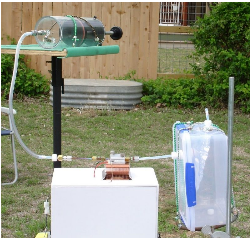
Figure S1. Collected air sample (during odor-cued air sampling into m-FEP bags (right)) is immediately transferred onto a sorbent tube (center). An operator uses manual syringe (left) and facilitates transfer of odor-cued sample collection from m-FEP bags to two sorbent tubes connected in series. Prototype Peltier cryo-trapping device (center bottom) shown clamped onto a Tenax TA packed fore-trap. Set to chill the fore-trap to \sim 2 °C to increase the trapping efficiency toward the high impact semi-volatile odorants.
