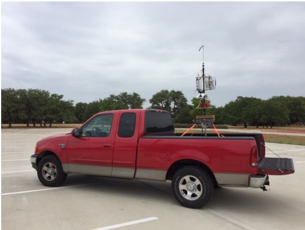
Figure S7. Truck-mounted prototype odor-cued grab sampling assembly. Added mobility is advantageous for transient odor events relocation and downwind air sampling.
