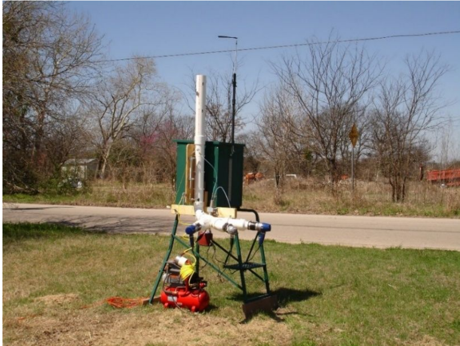
Figure S2. First-generation prototype scale-model transient odor event generator. The generator mixes three odorants and releases them through a single stack. A black wind strip-indicator mast shows the wind direction & velocity and informs the immediate downwind odor-cued sample collection.
