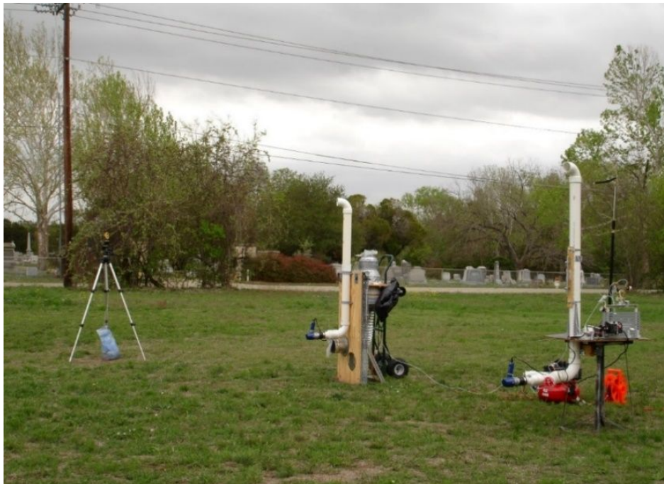
Figure S3. Integrated two point-source transient odor event generator systems [3]. A black wind strip-indicator mast visualizes the wind direction and velocity. To the right are the two contrasting odor point sources with vent stacks. To the left background is the tripod-mounted weather data station. Odor-cued sampling (not shown) occurs downwind to the left from the photo frame.
