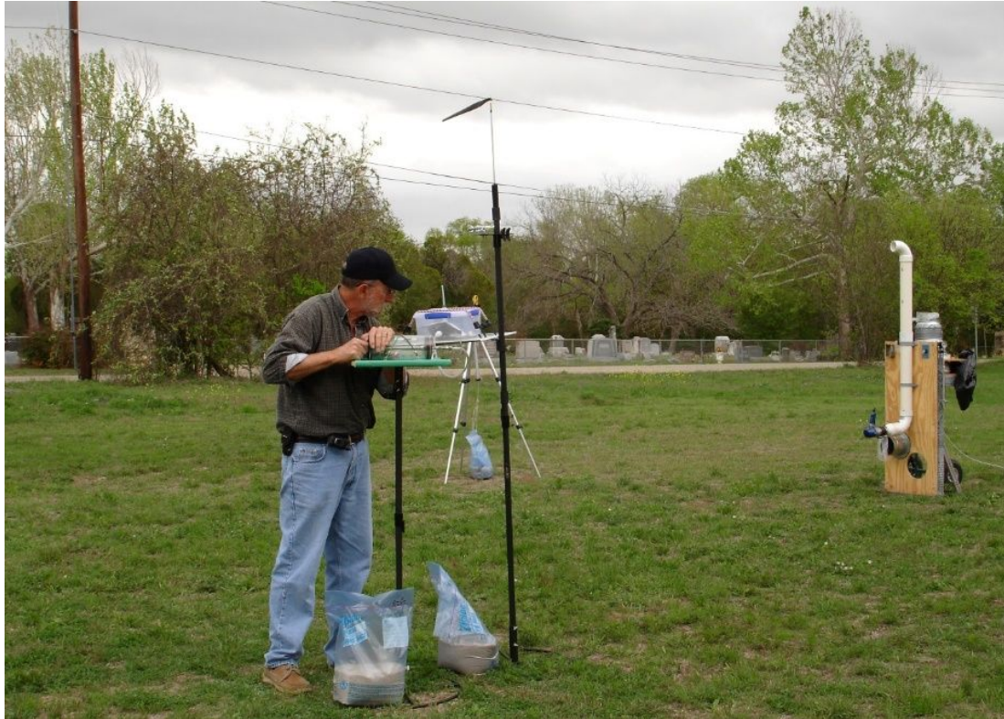
Figure S8: Odor-cued sampling of a transient odor event [3]. To the right is the left-most generator (early prototype) configured for controlled release of the naphthalene / chloroform odorant / tracer pair (shown in Figure S3; the second odor generator is to the right of the picture frame (not shown). The wind strip-indicator mast helps with the selection of downwind sampling location. The first author is shown awaiting the characteristic sensory cue for the targeted transient event. Utilizing the 1 L manual gas-tight syringe, the 1 L m-FEP gas sampling bags could be completely filled in 1-2 sec during the sensory cued events.
