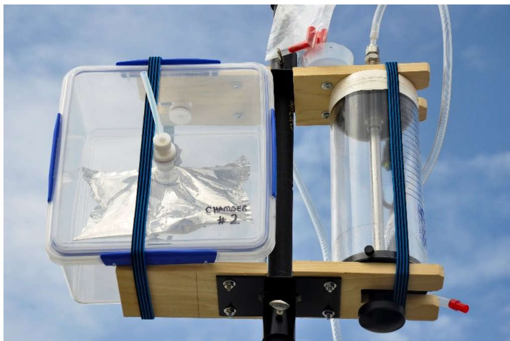
Figure S5. Second-generation prototype odor-cued grab sampling assembly: Close-up of syringe and sampling bag chamber 'cartridge' assemblies. Photo was taken 90 degrees (leftwise / counterclockwise) from ~ the operator's location on Figure S4.
