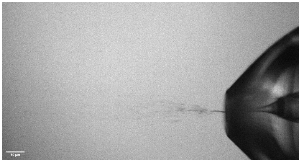
Figure S3: Imaging of the nozzle producing a spray with pulsed back light illumination. The total liquid flowrate is 55 \mu\text{L}/\text{min} and the nitrogen gas flowrate is 70 \text{mg}/\text{min} . A short jet rapidly breaks up into a heterogeneous and divergent spray.
