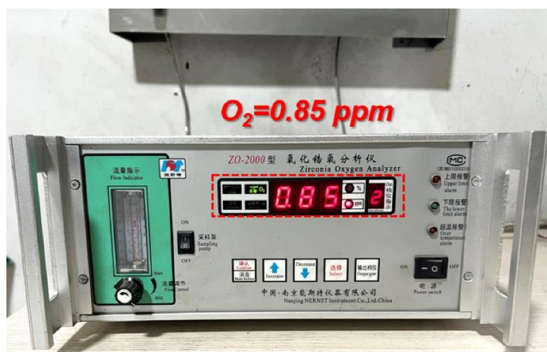
Supplementary Fig. 4 Photo of oxygen concentration after CO 2 RR tested by zirconia oxygen analyzer.
