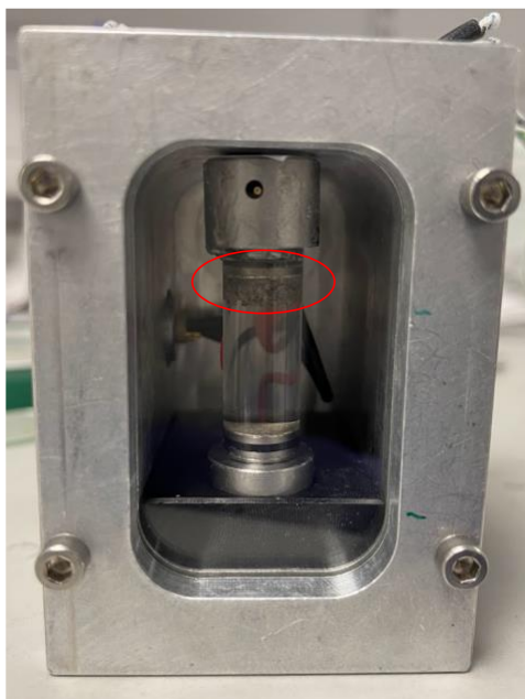
Figure S5: Photograph of the ORGA cell, post- cell operation, revealing the accumulation of dead/mossy lithium at the lithium plating side (red).
