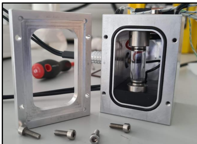
Figure S12: Photograph of the thermal chamber.
