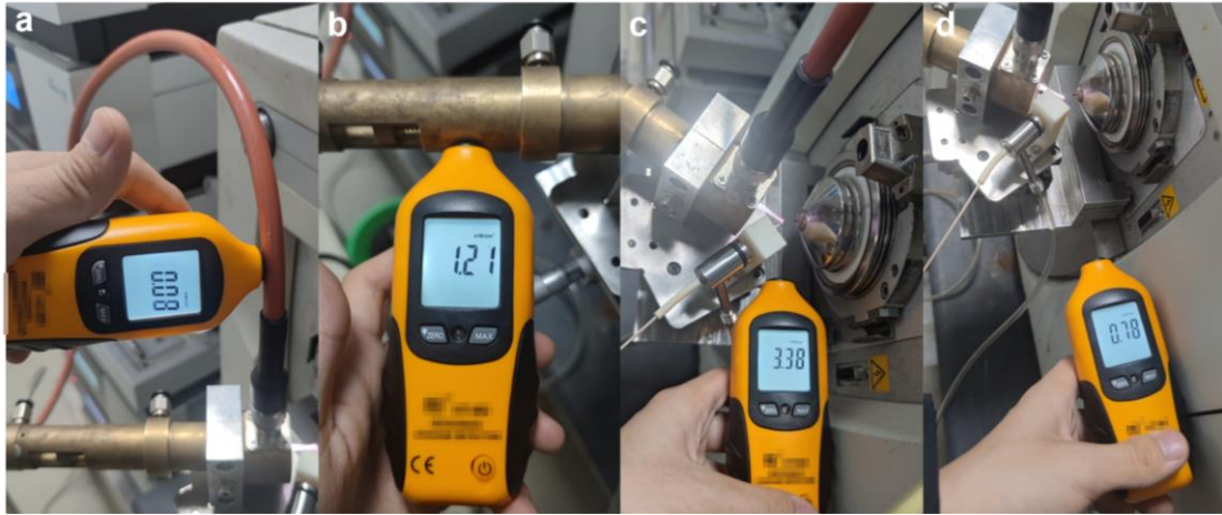
Supplementary Fig. 24. The microwave radiation levels were measured at various locations during the operation of WPMPI: a connecting line, b stick close to the main body, c 3 cm from the plasma tip, d 10 cm from the plasma tip.
