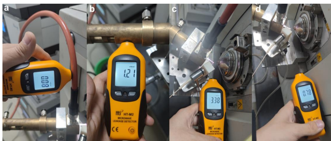
Supplementary Fig. 24. The microwave radiation levels were measured at various locations during the operation of WPMPI: a) connecting lines, b) stick close to the main body, c) 3 cm from the plasma tip, d). 10 cm from the plasma tip.
