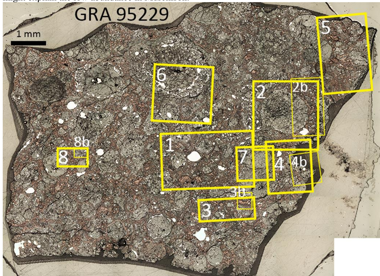
Fig. S4a. Reflected light image of the GRA 95229 thin section. Areas measured for sulfur XANES and XRF are shown in yellow squares. Sub-areas are shown by thinner yellow squares. The resolution of the coarse maps are 10 \mu\text{m}^2 to 20 \mu\text{m}^2 per pixel with a dwell time of 10-20 ms. The resolution of the fine maps are 3 \mu\text{m}^2 per pixel with a dwell time of 50-75 ms. The elemental sulfur and thiol peaks occur in areas 1, 4, 5, 8.
