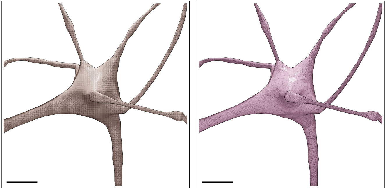
Figure S79: Wireframe visualizations of an L 5 _LBC neuron showing closeup comparisons between the highly tessellated surface mesh generated from the Voxel remesher (left) and the adaptively optimized surface mesh generated from the optimizer (right). Comparative quantitative and qualitative analyses of the meshes are demonstrated in Figure S80. Scale bars: 5 μm.
