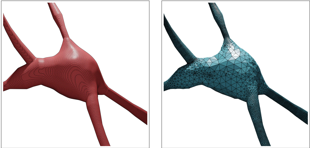
Figure S3: Surface mesh coarsening. The neuronal mesh generated from the Voxel remesher (left) is typically highly tessellated ( \sim 100k triangles). This mesh is re-tessellated using coarsening to create an adaptively optimized clone (right) – with \sim 68k triangles, where local regions with high frequency contain more faces than flat regions.
