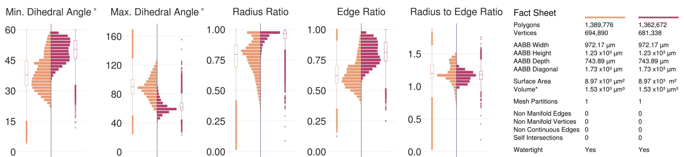
Figure S48: Comparative quantitative and qualitative analyses of the surface mesh models of the L4_BP neuron visualized in Figure S47.
