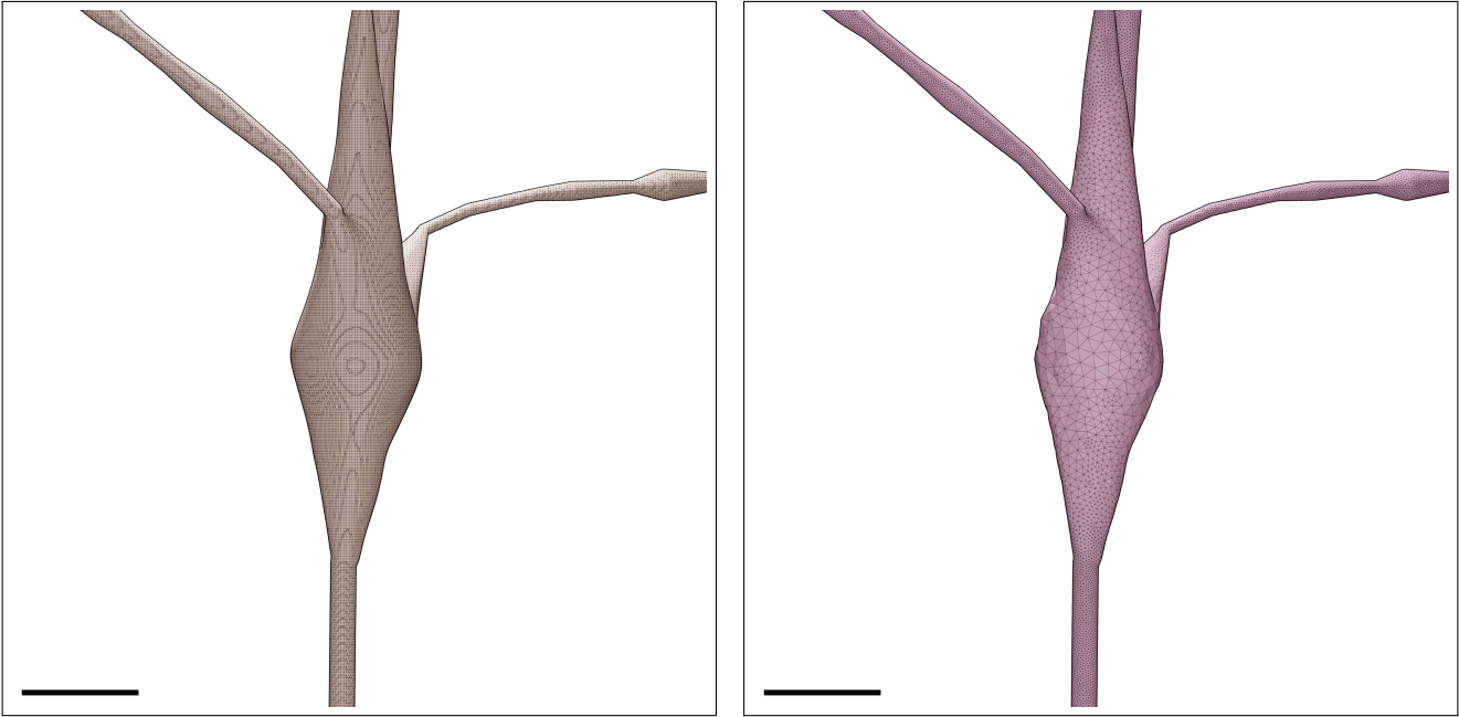
Figure S71: Wireframe visualizations of an L5_BP neuron showing closeup comparisons between the highly tessellated surface mesh generated from the Voxel remesher (left) and the adaptively optimized surface mesh generated from the optimizer (right). Comparative quantitative and qualitative analyses of the meshes are demonstrated in Figure S72. Scale bars: 5 \mu\text{m} .
