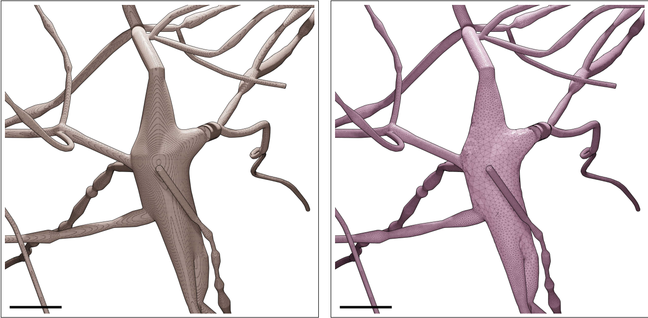
Figure S85: Wireframe visualizations of an L 5 _NGC neuron showing closeup comparisons between the highly tessellated surface mesh generated from the Voxel remesher (left) and the adaptively optimized surface mesh generated from the optimizer (right). Comparative quantitative and qualitative analyses of the meshes are demonstrated in Figure S86. Scale bars: 5 μm.
