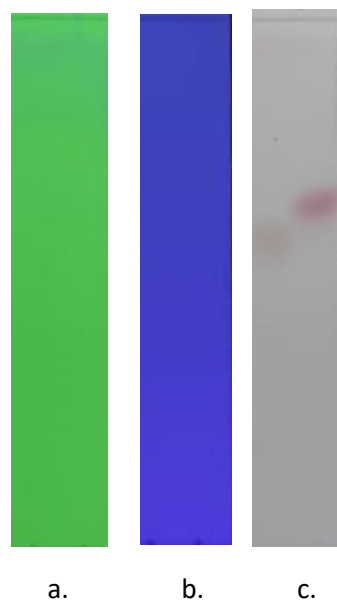
Figure S19 TLC profile of compounds 1 (left) and 2 (right) in Merck pre-coated silica gel 60 F 254 plates in n -hexane: DCM: EtOAc (7:2:1) at a. UV 254 nm, b. UV 365 nm, c. H 2 SO 4 spray
