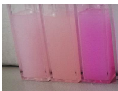
Figure S 3: Photograph of the used particle tracers in this study. From left to right: R6G-MSN@TiO 2 , SG-MSN@TiO 2 , RhB-MSN@TiO 2
