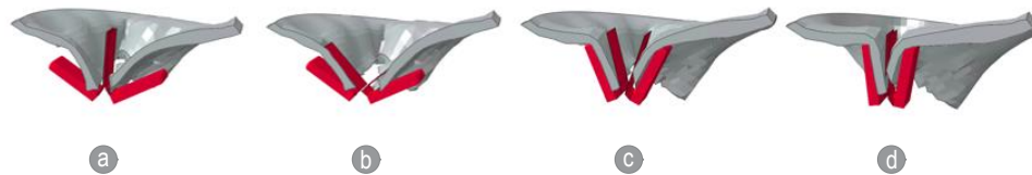
Figure A4: The coupled device-patient model illustrating the four steps used to (a) position, (b-c) deploy, and (d) release the clip.
