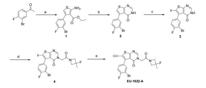
*Reagents and conditions:* (a) TiCl<sub>4</sub> (1M solution in DCM), ethyl cyanoacetate, pyridine, DCM, 0 °C – rt, o/n; (b) Et<sub>2</sub>NH, sulfur, THF, rt, 2h; (c) HCONH<sub>2</sub>, reflux, 16h; (d) K<sub>2</sub>CO<sub>3</sub>, KI, acetone, 80 °C, 16 h; (e) 1. Trimethylsilylacetylene, Et<sub>3</sub>N, Cul, PdCl<sub>2</sub>(PPh<sub>3</sub>)<sub>2</sub>, THF, 60°C. 2. TBAF, THF, 0°C, 30 min.
