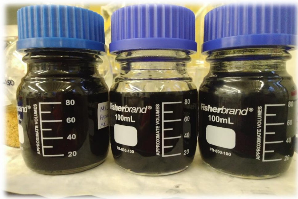
Figure S2. Concentrated solution of the delaminated (single-layered) Ti_3C_2T_x MXenes.
