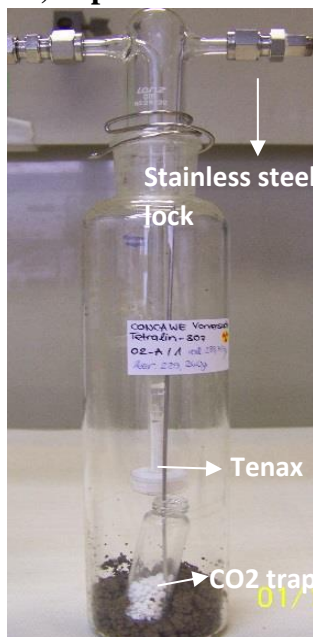
Figure S2 A Picture of test setup 1 used to test ^{14}\text{C} labelled tetralin during this study.
