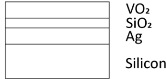
Figure S13. The schematic of the simulated filter.
