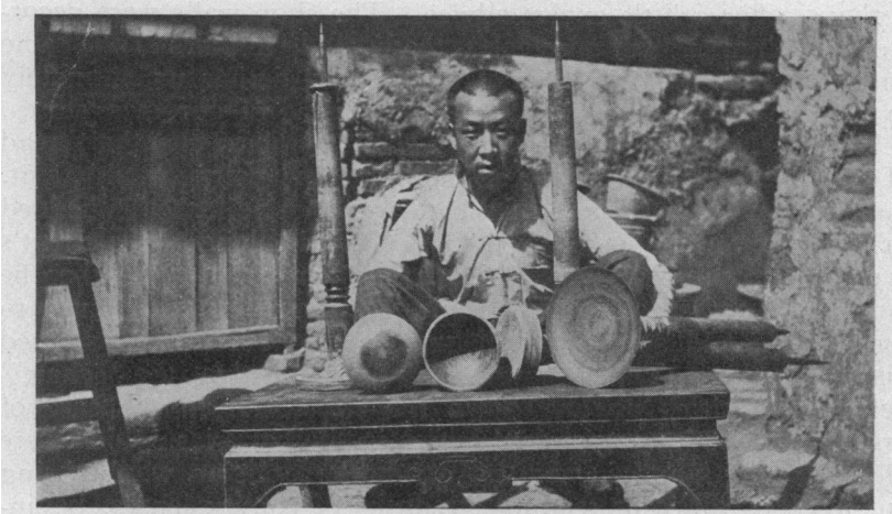
Ancient lens grinding tools.
