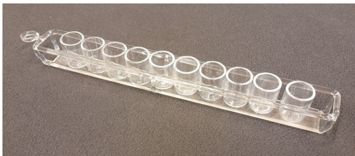
Figure S27. Cup holder and quartz cups used for the treatment of zirconia grinding spheres with sulfuric acid.
